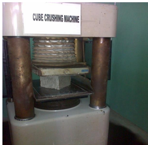
PLATE 1: Progress Photograph of Compressive Strength Test
